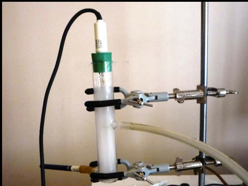
H-C T-113 trap with HI Flat Tip electrode
