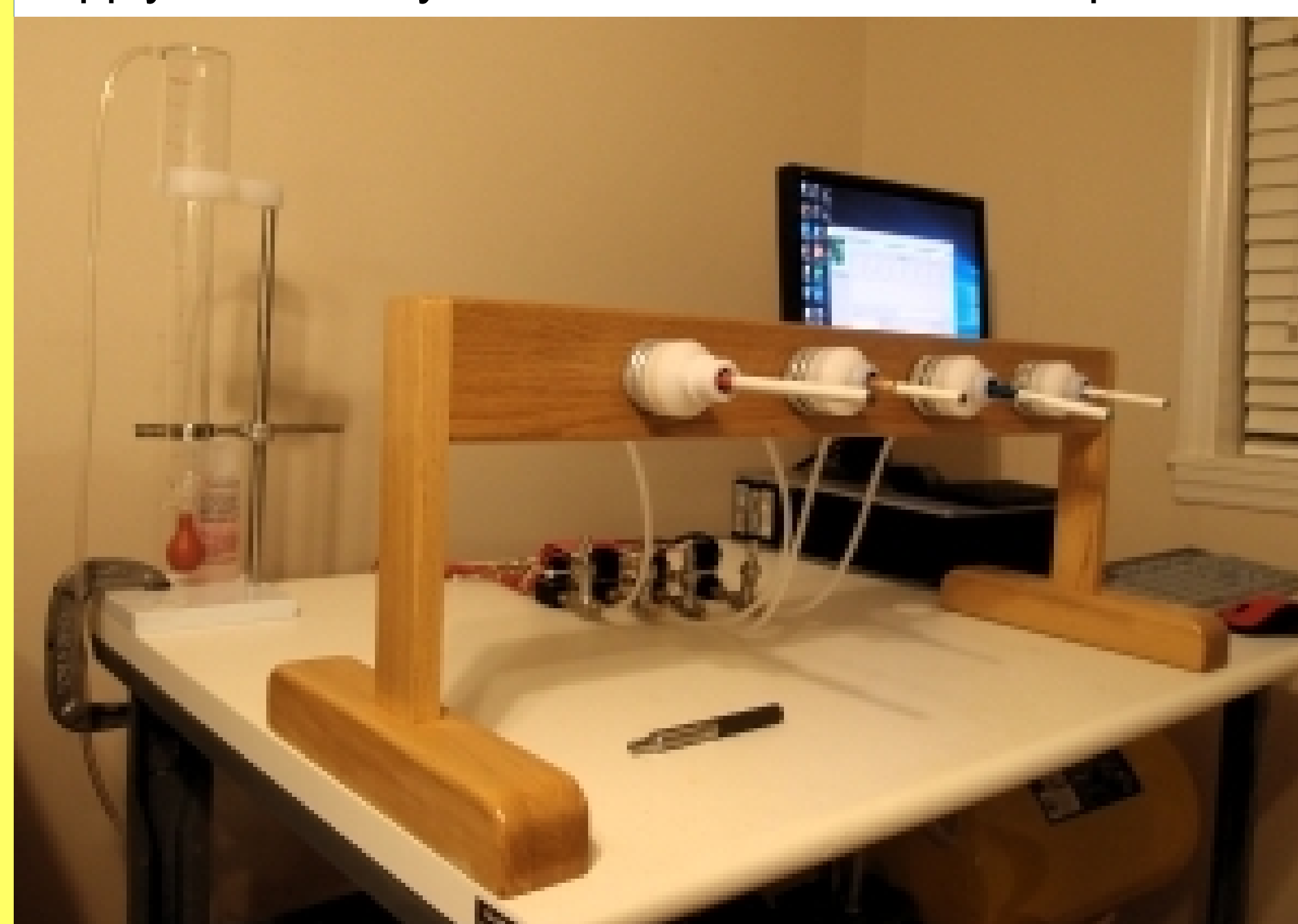
Figure 3 shows metering valve assembly with shutoff valves and solenoid valves.
