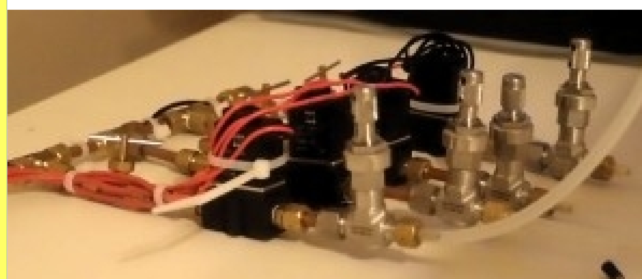
Figure 3 shows metering valve assembly with shutoff valves and solenoid valves.
